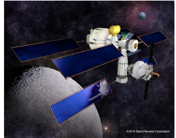
Concept image of SNC's habitation prototype based on its Dream Chaser cargo module.
